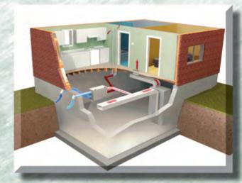
A continuous, balanced ventilation system brings in fresh air from the outside while exhausting stale air from the inside.
