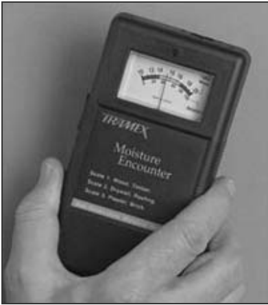
Figure 9. A Typical Pinless Moisture Meter
