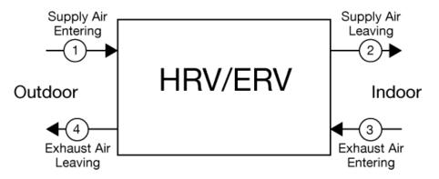
**External Static Pressure:** The total static pressure loss of the exhaust or supply system in the ductwork. In the case of the exhaust system, the total static pressure differential is the static pressure measured at point 4 minus the static pressure measured at point 3. The supply system total static pressure differential is the static pressure measured at point 2 minus the static pressure measured at point 1.
